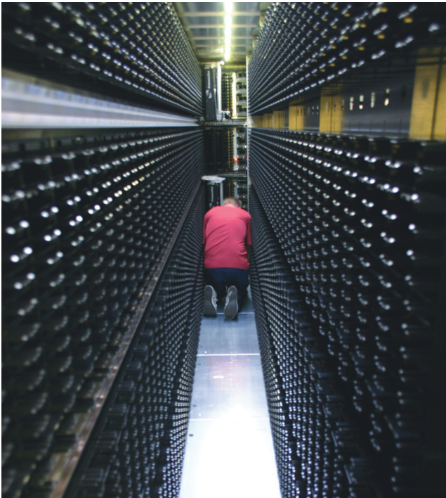
Figure 3 Inside one of the two corridors of an SL8500. Each ATL can house up to 10,000 tape cartridges.
